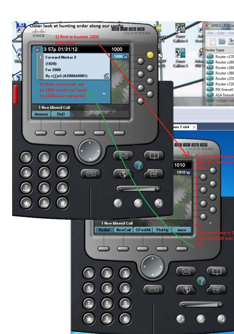
First number in hunt list is extension 1000 next hunted number is right from 1000 (it is 1010) because peer (circular) algorithm was configured using ephone-hunt 10 peer command. When hops reach 2 (two ringed extensions) final number 1000 take ringing line.
