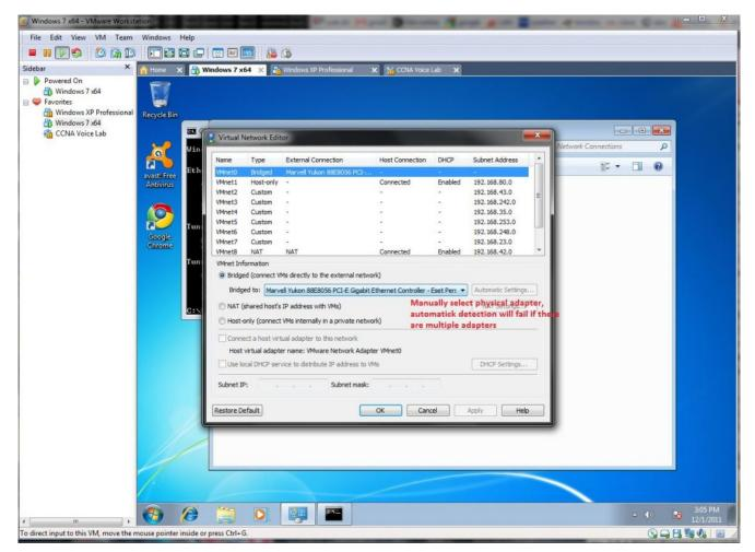
3) Configure IP address in hosted PC (in our scenario we used 172.16.0.15/24 and 172.16.0.1 as default gateway) -address assignment must be derived from your home network config – CME router and ephones are in this simple scenario in same subnet.
