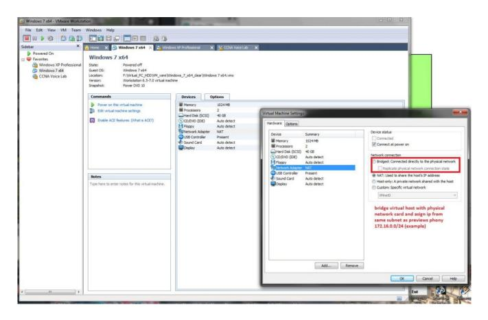
2) If you have more than one installed network adapter (WiFi, second network card, or virtual card of VMware) you must manually select appropriate bridging adapter as hosting client physical adapter (better is if you check it)
