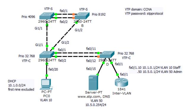
Scenario consist of 4 switches. Root bridge role is determined by spanning-tree vlan 1, 10, 50 priority 4096 command for switch A. For VLAN information consistency is used proprietary VTP protocol with VTP domain: CCNA and password: stpprotocol. For redundancy of server roles in VTP two switches A and B are configured as VTP servers. Inter VLAN communication establish router on a stick Inter-VLAN.
