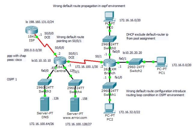
Network topology consist of central router (act as boundary between office network and WAN) and one branch router (for simplicity is there only one branch router). All end devices are on separate networks and private address space is in use in internal network. Wrong default route
