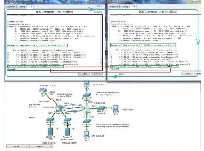
Now is time correct our mistake. What we need to do? At first you must remove wrong default route. There is no way how to change existing static route. First remove wrong route with command
