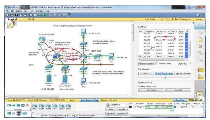
Wrong default route lead PDU to its origin and Branch router loop back to central router with default route. L3 PDU contain mechanism how to break endless looping of PDU — TTL in data packet header is decreased after L3 routing to appropriate interface as you can see on next picture (PDU examination in cisco packet tracer — simulation mode).
