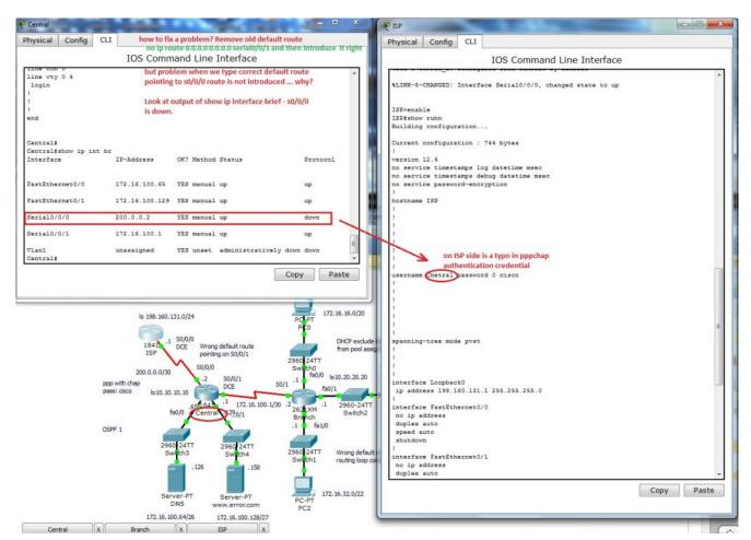
Default route is now correct but can we establish a connection between end devices on office network and ISP? Fire ICMP packet to destination nework 198.160.131.1. Packet can reach ISP router but then is discarded because no translation to public network have not been made. We are closer to our goal, data re well routed but address translation on private network boundary must be established.
