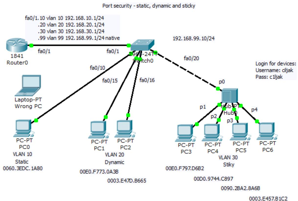
Network topology consist of router acting on stick and switch. Port security is configured sticky for 10 mac address for port 20 to 24 with commands:
