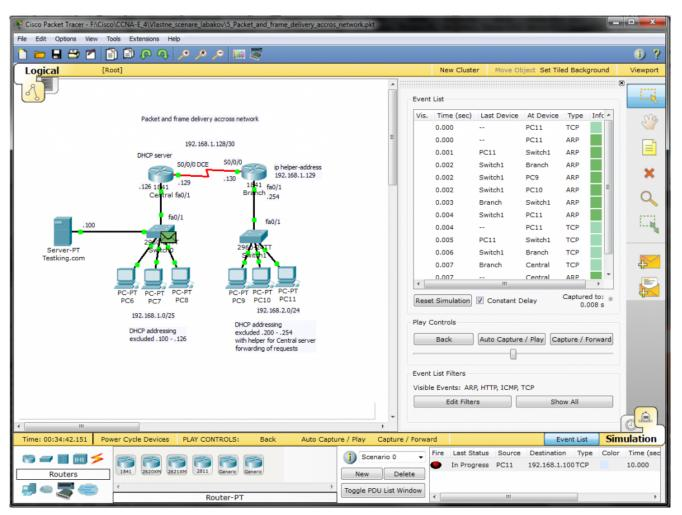
After appropriate time used for PDU propagation across network (and ARP caching for L2 encapsulation), PC11 can send frame to Branch fa0/1 interface that act as a default gateway. You can scroll event list and look at PDU emitted by PC11 after ARP process as it show next picture.
