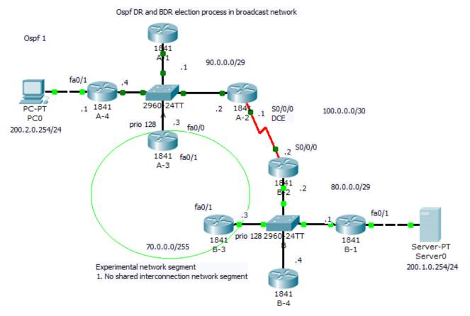
For best route selection process from network 200.2.0.0/24 PC0 to Server0 in network 200.1.0.0/24 use command show ip route on A-4 and B-1 routers. How are cumulative bandwidth increased
