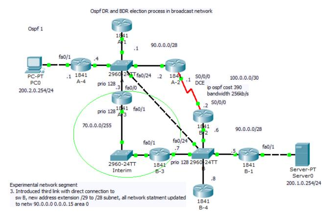
Explanation of DR, BDR selection and cumulative bandwidth calculation for best path is on next picture, Router -IDs are included in picture (no lo interface and router -id command was issued on any router — then higher ip of any active interface is used for ospf router-ID derivation).
