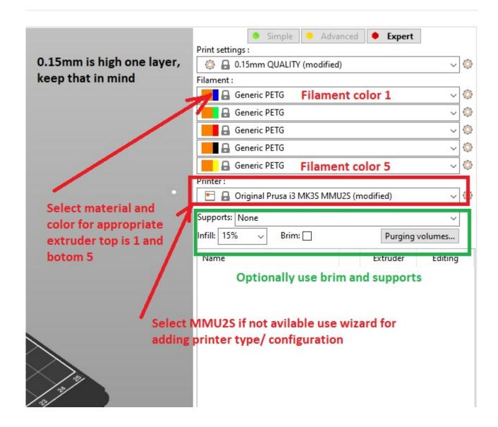
Before next step, we must look at our model and recognize what part is base on top of their are other parts added. In our exmple it is orange part. This part can be drag and drop into space of slicer. Other parts are added on the top and the create final MMU composit.
