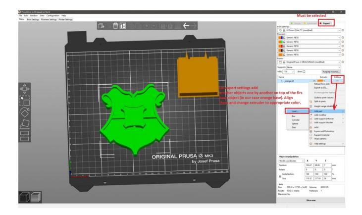
After adding first part, use rightclick on selected part and change extruder to appropriate color. Repeat his steps — add, change extruder to appropriate color until last part of model.
