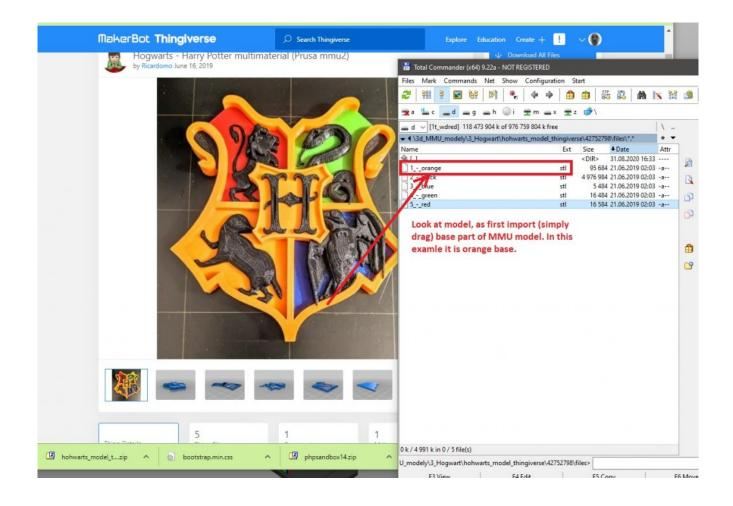
After import of first (base) orange part, we must rightclick on the object and select extruder with appropriate filament, in our case it is extruder 5 with orange filament.
