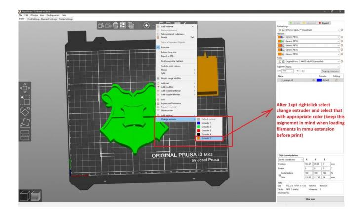
In next step we must switch on expert settings and on object pane (right bottom layered part) we click on add option (with sign + in circle). Next select add part and load one of remaining parts from disk. Our downloaded files are named by color in spanish, but it can be recognized or translated and refered with picture of modell on thingiverse.
