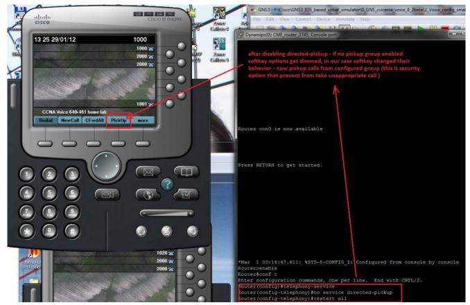
Much more control to pickup of ringing ephone introduce pickup groups. We can use pickup-group command in config ephone-DN. In our scenario it is
