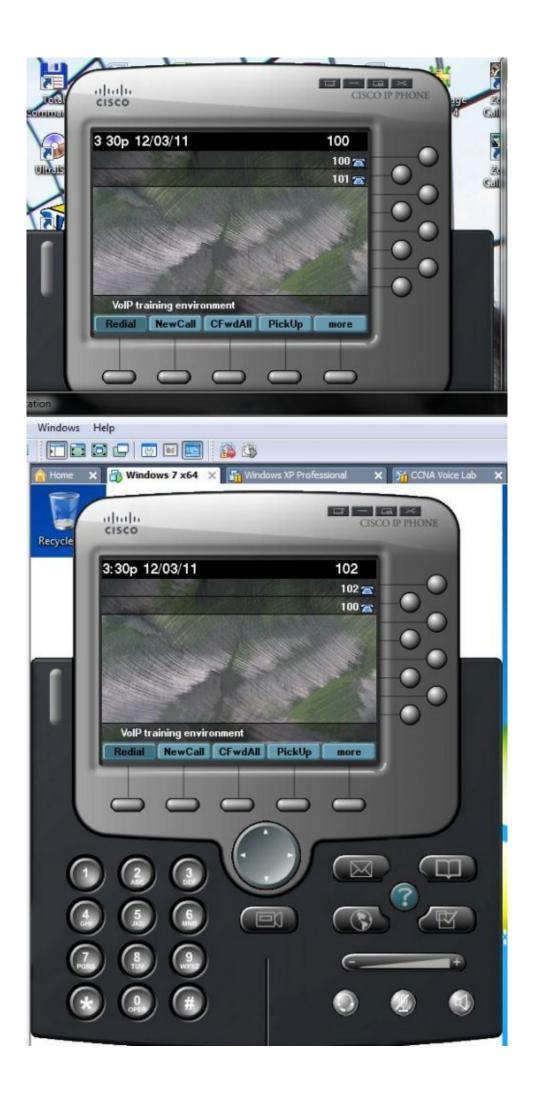
3) Watch line activity during call on upper ephone (watch line is second line on bottom ephone that monitor upper ephone line active — call to 101 or 100 number)
