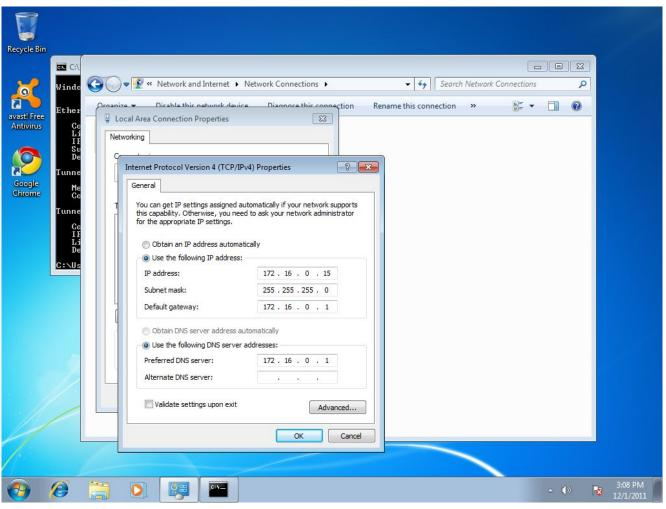
4) *Verification of local stack* and connectivity with CME router 172.16.0.20/24 from hosted PC (installed in VMware)
