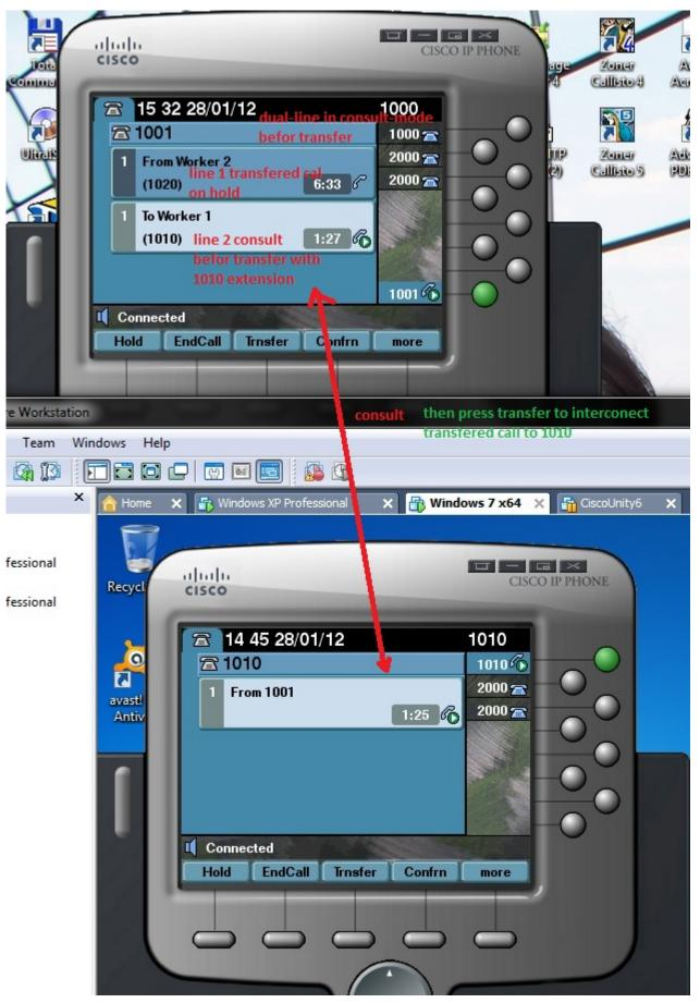
When consult is at its end i can press Trnsfer softkey for second time that definitive transfer call from my ephone with extension 1001 to 1010 extension. As you can see call is transferred from 1001 to 1010 and all communication is now only between 1020 (initiator of call) and 1010 (call was transferring from 1001 to new extension 1010).
