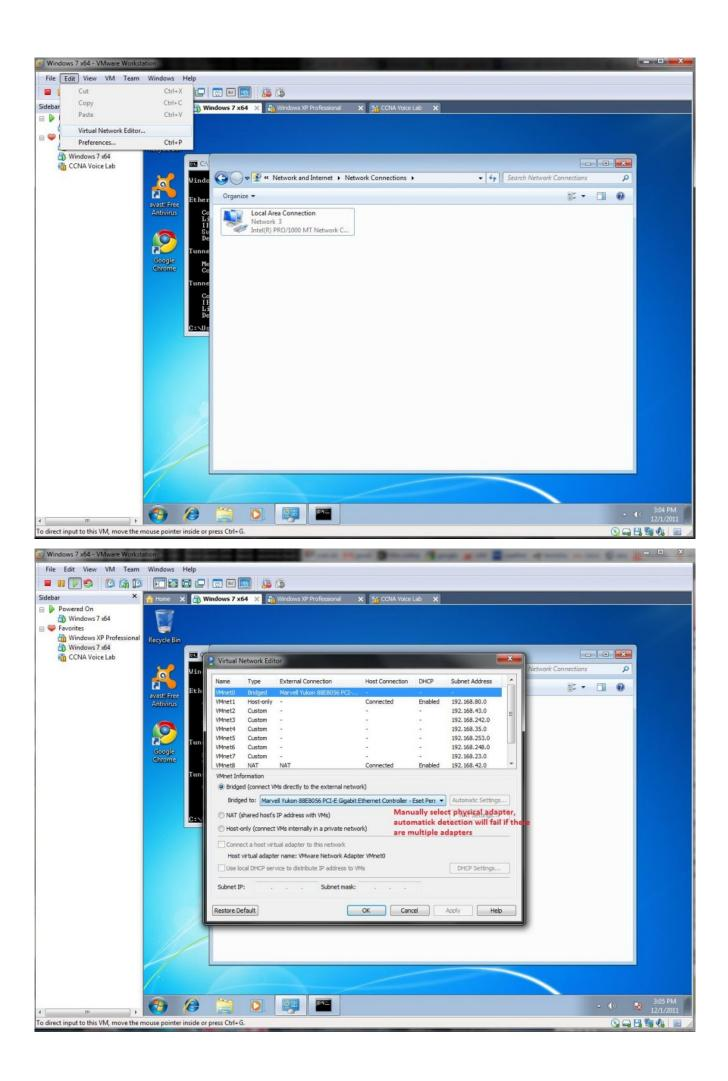
3) Configure IP address in hosted PC (in our scenario we used 172.16.0.15/24 and 172.16.0.1 as default gateway) -address assignment must be derived from your home network config – CME router and ephones are in this simple scenario in same subnet.
