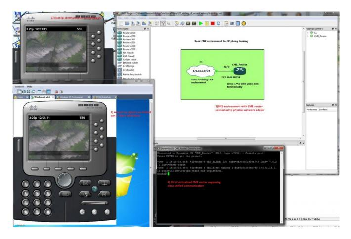
Ephone at top is installed in hosting PC with 172.16.0.10/24 IP, bottom ephone installed in hosted (virtualized) PC with 172.16.0.15/24 IP and GNS emulated cisco IOS with telephony service has its fa0/0 interface configured with ip 172.16.0.20/24 and acting as CME router (voice gateway).
