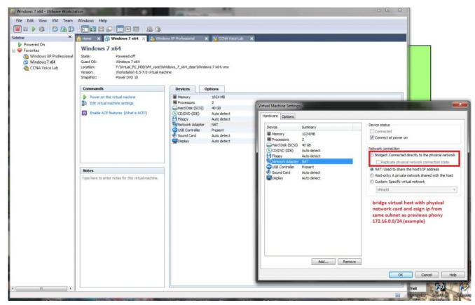
2) If you have more than one installed network adapter (WiFi, second network card, or virtual card of VMware) you must manually select appropriate bridging adapter as hosting client physical adapter (better is if you check it)
